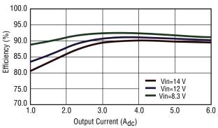
Fig. 5 Efficiency vs. Output Current ( $V_{out} = 3.3 V_{dc}$ )
