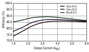
Fig. 3 Efficiency vs. Output Current ( $V_{out} = 1.8 V_{dc}$ )
