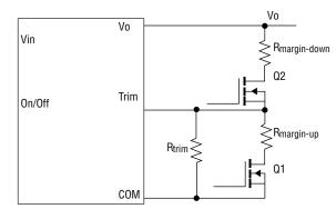
Fig. 26 Circuit Configuration for Margining Output Voltage
