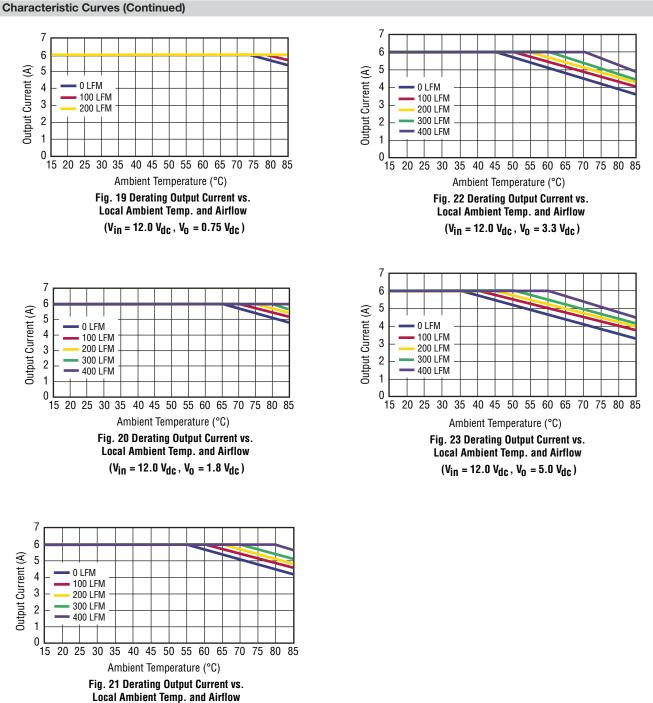
$(V_{in} = 12.0 V_{dc}, V_0 = 2.5 V_{dc})$
