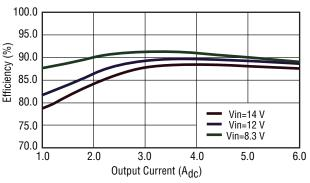
Fig. 4 Efficiency vs. Output Current (Vout = 2.5 Vdc)
