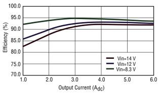
Fig. 6 Efficiency vs. Output Current ( $V_{out} = 5.0 V_{dc}$ )
