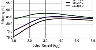
Fig. 2 Efficiency vs. Output Current ( $V_{out} = 1.5 V_{dc}$ )
